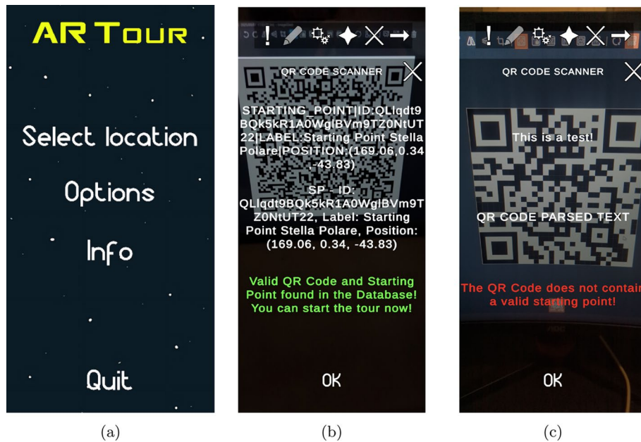
Fig. 2 ARtour interface illustrating the localization workflow: main menu and location selection (left), successful parsing and validation of a QR code associated with a Starting Point (center), and error notification when the scanned QR code does not correspond to a valid Starting Point (right)
